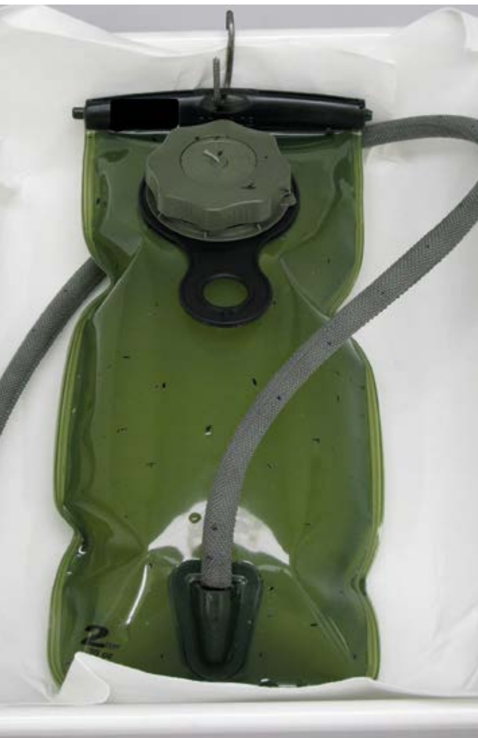
Figure 2: Hydration system loaded with HD. It consists of a drinking bladder, a drinking tube and a mask adapter (not shown here). All components are being tested.
